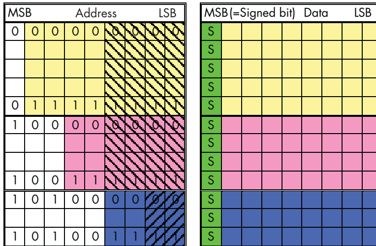
Figure 13. Substitution Matrix Storage Structure in Memory
